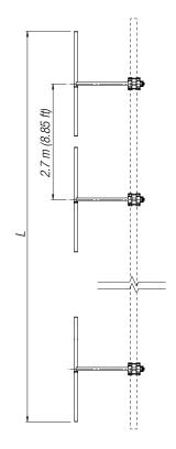
Total Antenna Height (L) is subject to change according to requirement. Custom designed antennas meeting special requirements such as specific azimuthal pattern, different gains and custom power input are available upon request.
