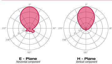
WORKING BAND: 87.5 - 108 MHz BANDWIDTH: VHF band FM GAIN: 7.5 dBd (9.7 dBi) VSWR: ≤ 1.2:1 (-20.8 dB) POLARIZATION: Vertical or Horizontal IMPEDANCE: 50 Ohm balanced HALF POWER BEAMWIDTH: E-Plane - 70° H-Plane - 64° LIGHTNING PROTECTION: All metal parts DC grounded including inner conductors AVAILABLE VERSION AND CODE: ADP0202415 - EIA 7/8" - max 5000W rms ADP0202416 - DIN 7/16 female - max 3000W rms ADP0202417 - N - max 800W rms
