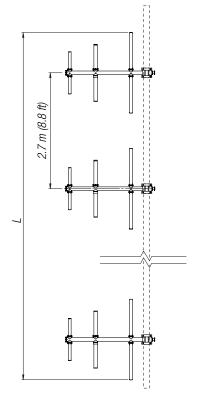
Total Antenna Height (L) is subject to change according to requirement. Custom designed antennas meeting special requirements such as specific azimuthal pattern, different gains and custom power input are available upon request.
